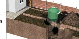
installation of the BIODIGESTER, you must establish the water table at the intended location. This must be the depth of the winter (peak) water table. Once you ascertain its depth, select one of the two methods of installation detailed below - "Wet Ground" or "Dry Ground".
