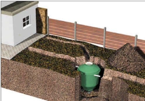
Before you commence installation of the BIODIGESTER, you must establish the water table at the intended location. This must be the depth of the winter (peak) water table. Once you ascertain its depth, select one of the two methods of installation detailed below - "Wet Ground" or "Dry Ground".
